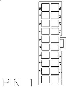
FIGURE 37 - REAR VIEW OF CABLE CONNECTOR
