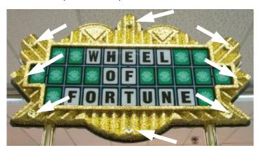
2. Remove the bolts that hold the inside wood housing together.
