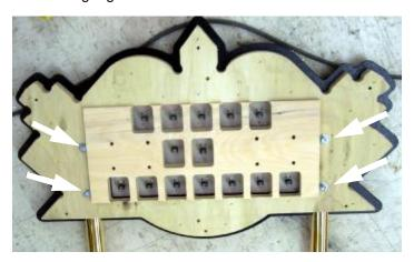
3. Remove the main p.c. board by removing the screws and connector that hold it in place.
