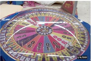
DIFFICULTY – This makes it easier or harder to hit the "spin zone" target. This will make the wheel spin less or more often. The wheel is set up with a difficulty of "6" from the factory. This allows the average player to spin the wheel about once every 20 times.
