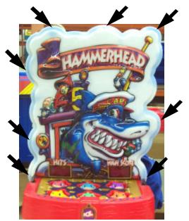
3. Using a Phillips screwdriver, remove the four screws that hold the board in place.
