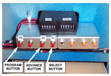
3. To enter programming, press the Program button once. Each programming mode is identified by the "LED lit" (mode 1, 1st LED lit, mode 2, 2nd LED lit; etc.). To exit programming, press the Program button once.
