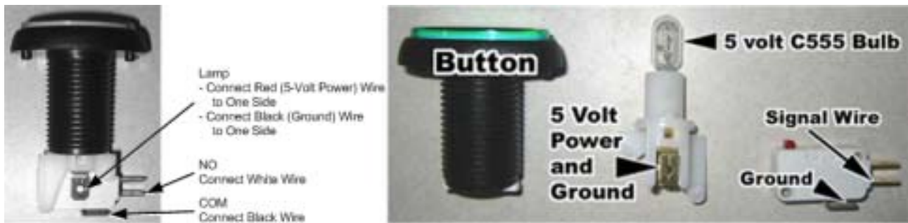
Figure 32. Replacing Button Lamps
