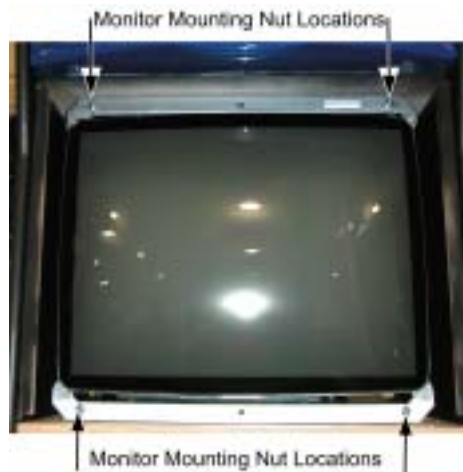
Figure 37. Monitor Mounting Nut Locations
