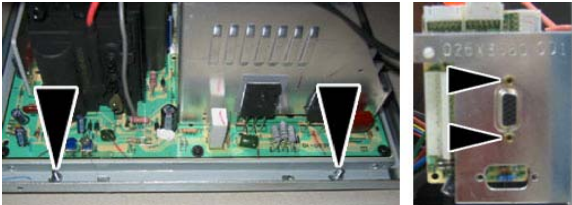
Figure 38. Removing the Monitor PCB Mounting Hardware
