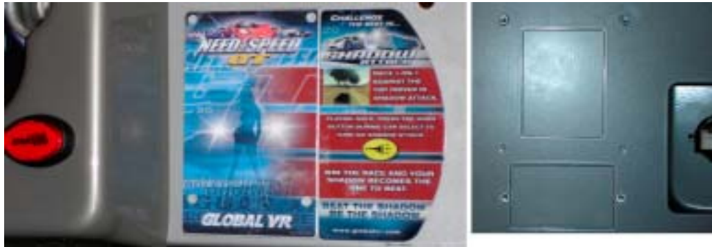
Figure 16. NOS Button and SmartCard Reader Location (Deluxe Cabinet)
