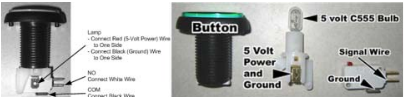
Figure 53. Replacing Button Lamps
