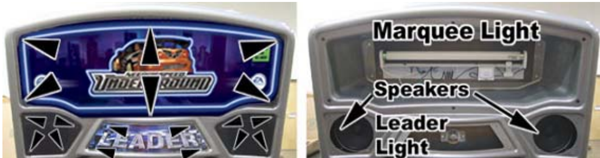
Figure 70. Accessing the Marquee Light, Leader Light, and Speakers
