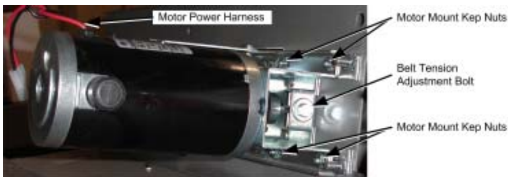
Figure 52. Servicing the Steering motor
