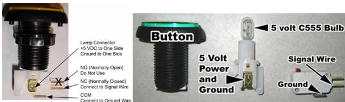
Figure 22. Replacing Button Lamps
