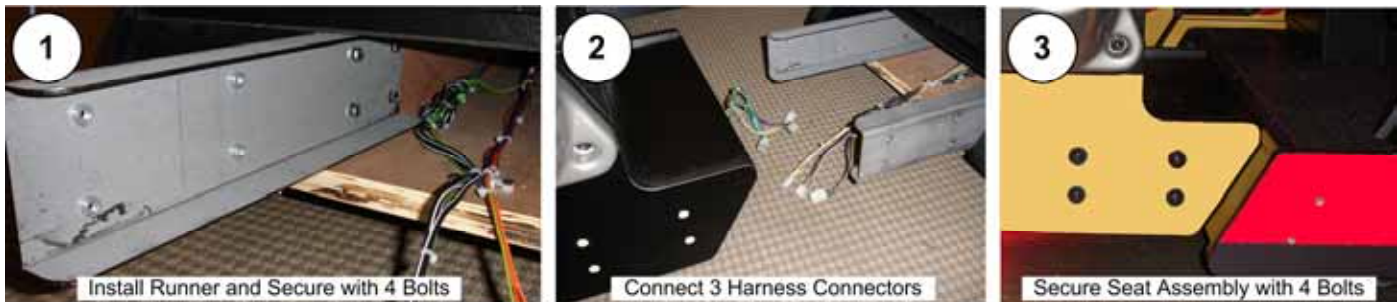
Figure 3. Installing the Seat Runners
