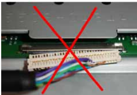
Figure 31. Connecting the LCD Control PCB Harness
