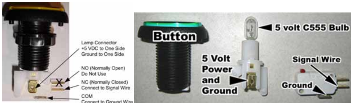
Figure 19. Replacing Button Lamps
