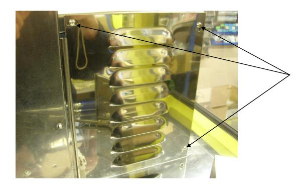
3. Remove 4 screws identified in the picture below and move the cover to the left to expose the water nozzle. On some machines there is a  $5^{th}$  screw at the top rear.
