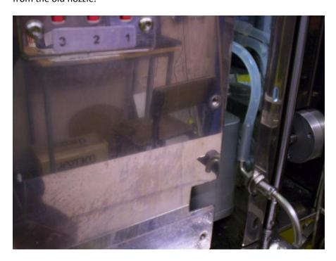
5. Fit the flexible hose to the end of the new water nozzle with the internal countersink.
