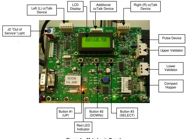
Figure 1 – Main Logic Board
